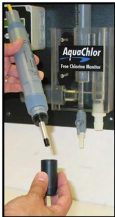
5: Assemble the membrane cap back onto the sensor head. Screw the cap on slowly until it seats against the gasket at the base of the sensor head. Some excess electrolyte will drip out of the top of the cap as it is threaded onto the sensor head.
