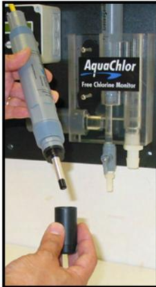
2: Unscrew the membrane cap from the sensor head.
