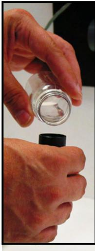
4: Fill the membrane cap with Free Chlorine Electrolyte (PN: RDOK9). Fill it up to the step just below the internal threads inside the membrane cap.
